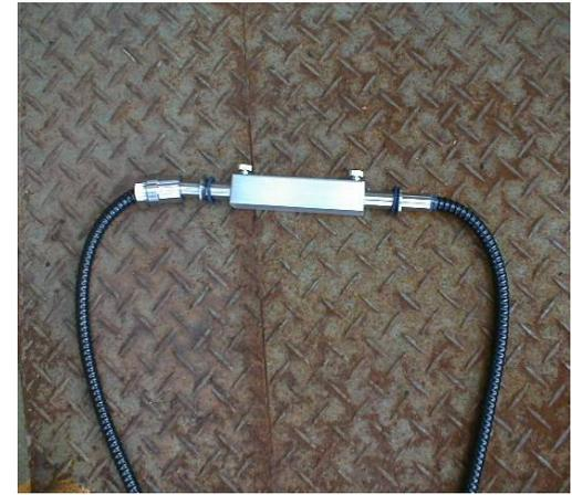
**It is possible to connect to the calibration box by removing optical fiber cables from detector head even if flue gas flows.**
