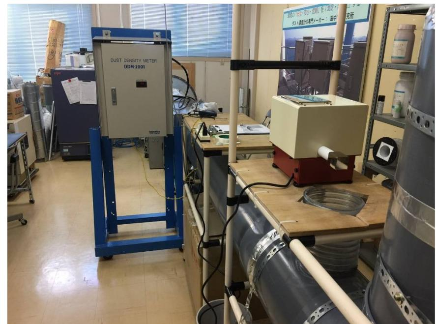
Duct : Straight length is 4,225mm , diameter is 300φ
