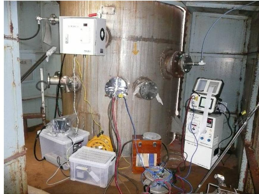
Test by isokinetic sampling (JISZ8808)
