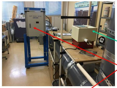
Test for getting correlation coefficient between isokinetic sampling method and automated dust monitor.
