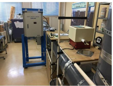
Duct: Straight length is 4,225mm, diameter is 300φ
