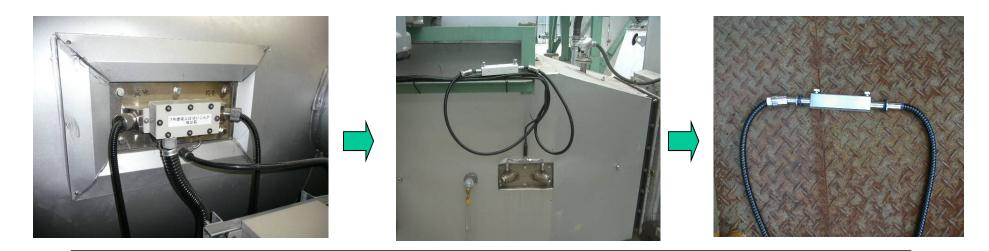
It is possible to connect to the calibration box by removing optical fiber cables from detector head even if flue gas flows.
